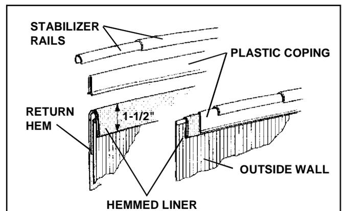
Pull liner up and over pool wall. Make a hem along the top edge of the liner. Pull hem back over the top edge of the pool wall as shown so it hangs over top edge of pool wall by about 2". Install plastic coping by pushing it all the way down to overlap pool wall and liner as shown. Make sure the plastic coping is butted end to end. Install enough coping to cover two top rail lengths centered where you removed the top rails in Step 21.
