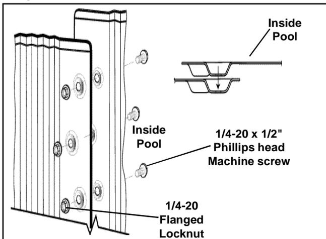
Bring wall ends together in center of bottom connector. If wall ends do not meet, adjust all bottom rails in or out uniformly as required. Do not make the total adjustment with one or two bottom rails. Remove stabilizer rails in the areas above the pool wall ends.
