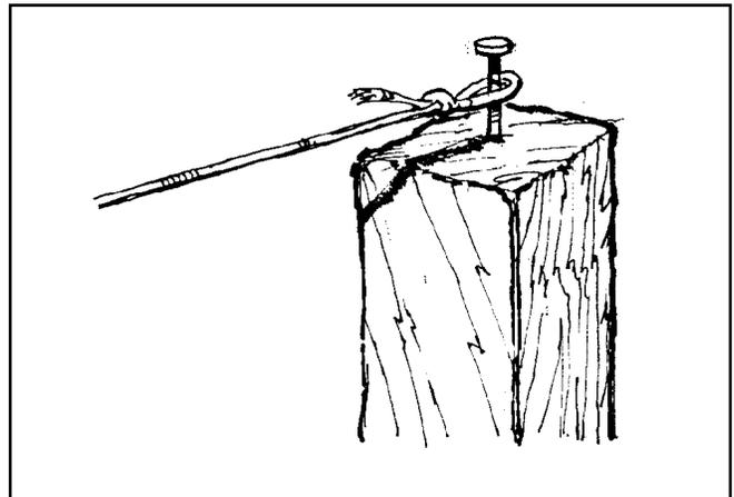
Stake the center of the pool area. Drive a 2 1/2" long nail into top of stake as shown. Tie a loop in one end of a piece of twine at least 12" longer than your pool clearance radius. Slip loop over exposed head of nail in center stake as shown.
