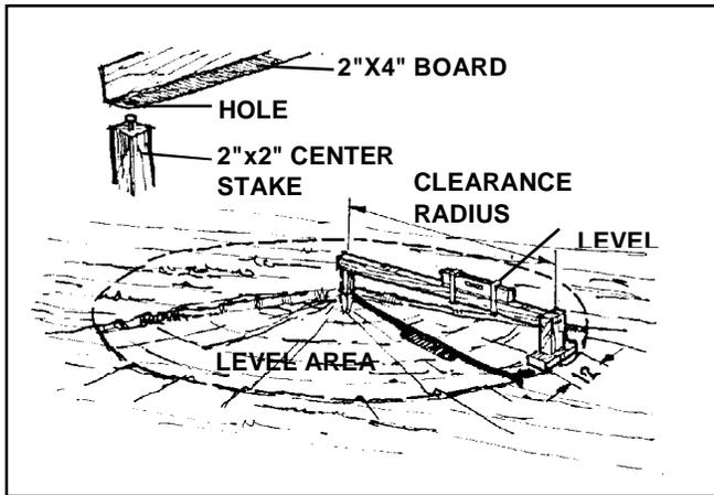
A homemade leveling device can be made:
