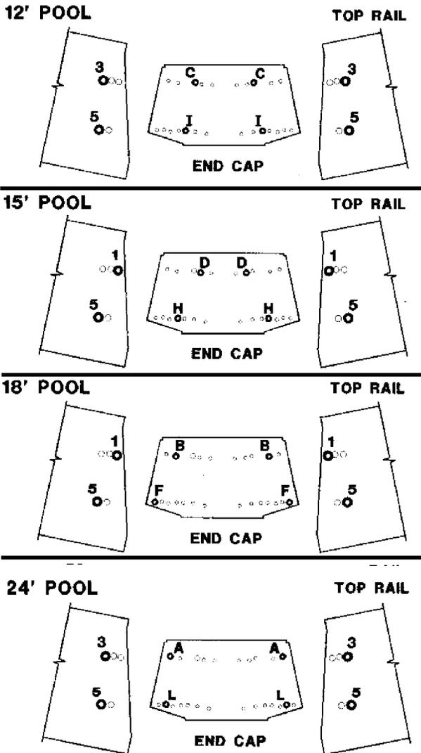
Attach the top rails to the end cap using four (4) 3/8" long sheet metal screws.
