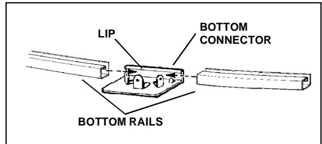
The bottom rails slide under the lip of the bottom connector. The ends of the bottom rails meet in the center of bottom connector. Do not bend or distort bottom rails. Keep rails free of dirt.
