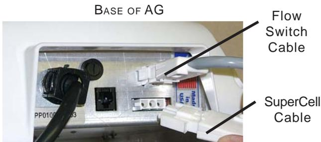
A Flow Switch Jumper has been provided with your AG system to disable the water flow switch when used with the 75093 and 75092 manifold systems. These manifold systems do not use a flow switch to monitor water flow. Do not use this jumper with the 75094 "Inline-cell manifold system".
